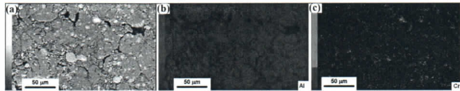
Figure 17. (a) Microstructure of Al-7.5Cr consolidated sample, chemical mappings of (b) Al and (c) Cr.
